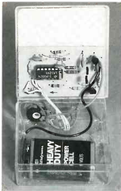
FIG. 5—EXAMINE THE COMPLETED board for shorts, opens, and cold solder joints before installing it in a plastic case.
